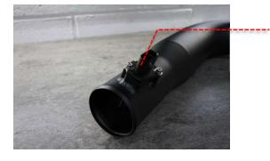
10 Install the Revo intake pipe using the 60-80 hose clamp on the Revo elbow hose (loosely tighten until ready). Next, bolt the Revo intake pipe to the engine using the M6 bolt, M6 washer, M6 lock washer and M6 black nylon spacer, as shown. Note: D0 NOT OVER TIGHTEN THE BOLT INTO THE PIPE, ONCE IT NIPS UP TO THE LOCK WASHER THERE WILL STILL BE MOVEMENT IN THE PIPE WHICH IS HOW IT SHOULD BE, THIS IS NOT A SOLID MOUNTED POINT!
